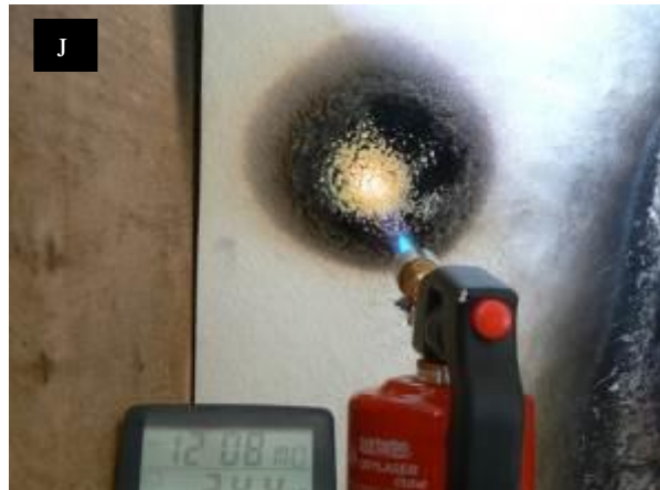
After 8 minutes the char barrier glowed yellow/white and the smoke omission noted earlier had stopped
