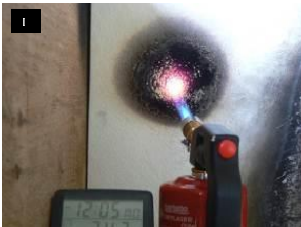
After 5 minutes the char barrier glowed red and some smoke was observed from the reverse of the panel
