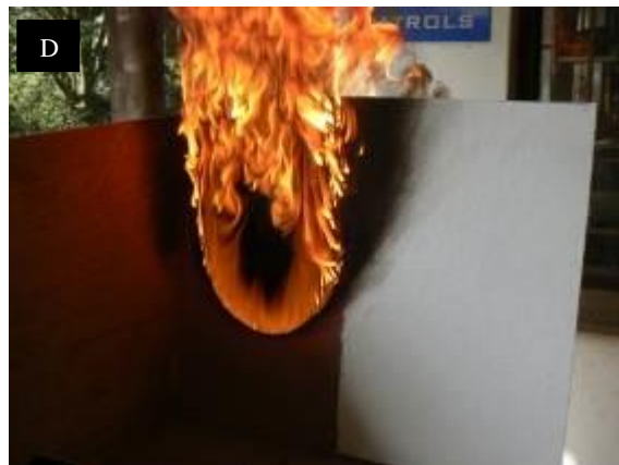
At 1 minutes 10 seconds the panel was burning out of control and had burnt through the sample
