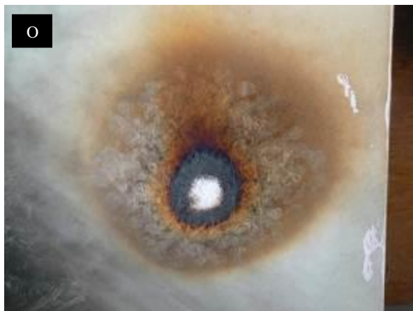
The untreated side was undamaged and did not burn through or rupture the surface. No excessive smoke was emitted during the test
