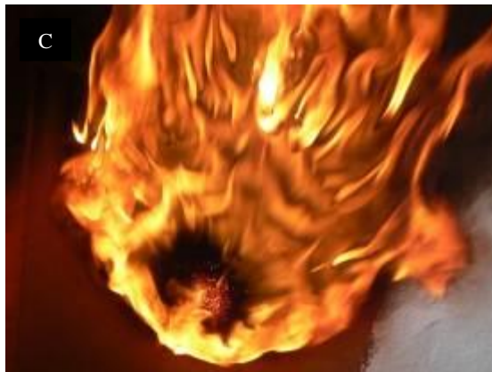
After 30 seconds the flames spread over the panel and burnt vigorously
