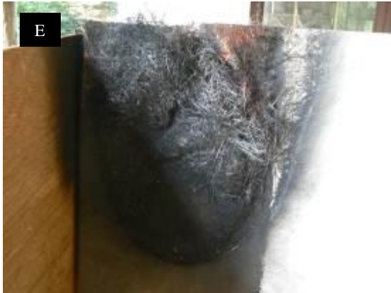
The sample had lost its structural stability due to the resin having burnt away exposing the glass fibre
