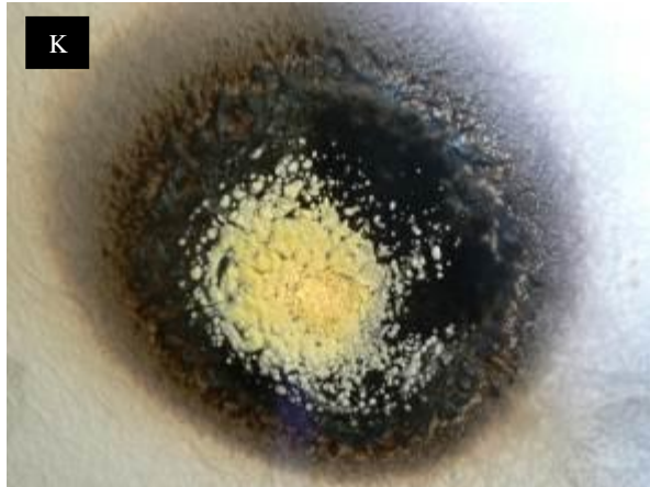
A close up of the char barrier after 30 minutes
